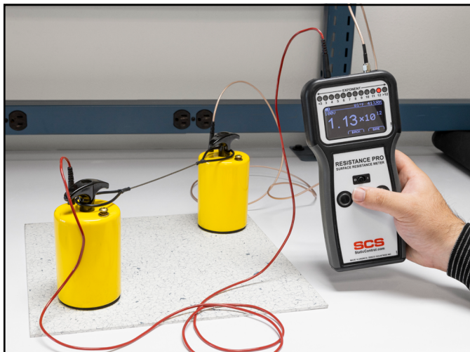
Figure 12. Measuring the Resistance Point-to-Point (R tt ) of a floor tile
